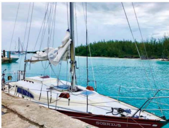
Slab reefing is performed at the mast, as is raising the sails via winches on both sides of the mast.
