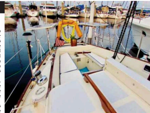
The reverse-wineglass transom is pinched in and thus the cockpit is narrow, ideal for offshore sailing. The cockpit benches are about 6.5 feet, just long and wide enough for most people to lie down in.
